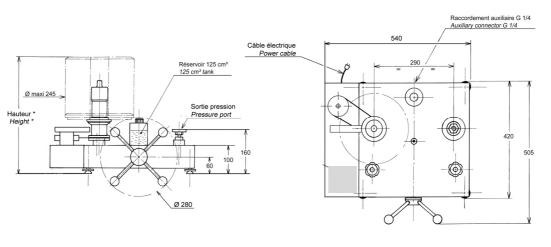
Height with standard set of weight : (bar, kPa) : 450 mm (PSI) : 465 mm
